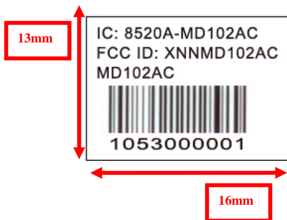
Figure: Example MD-102AC Labeling for FCC Approved Modules
