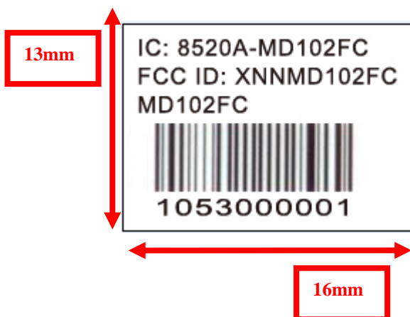
Figure: Example MD-102FC Labeling for FCC Approved Modules
